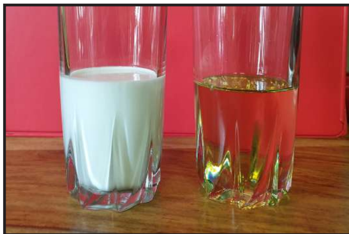
Deltaforce 100 (left); Eraditick 250 (right) illustrating the difference between SC (soluble concentration) and EC (emulsifiable concentration).
